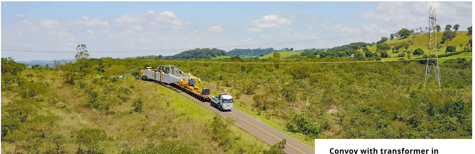
Convoy with transformer in side girder bridge in Cristais Paulista, Brazil
