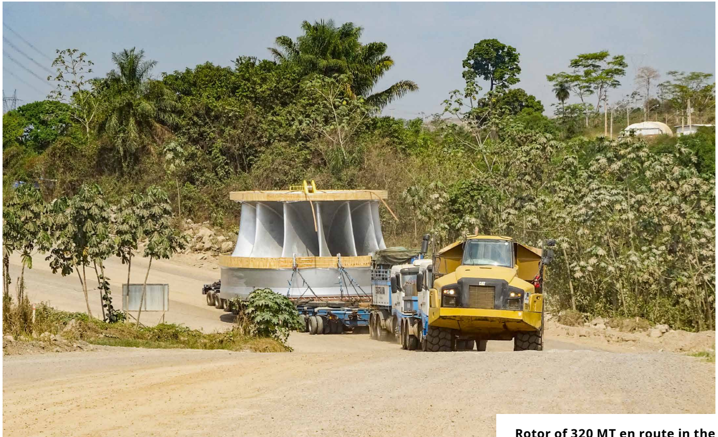
Rotor of 320 MT en route in the remote area of Xingu, Brazil
